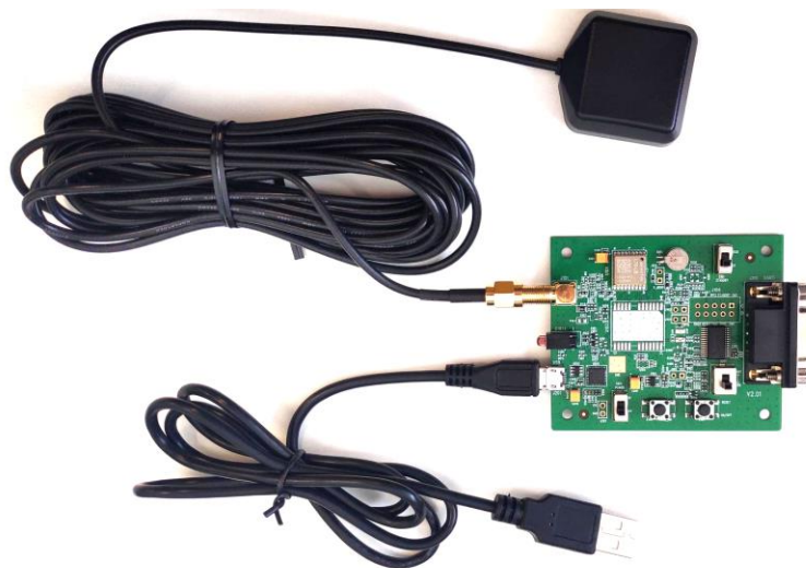
Figure 2: EVb and Accessories Assembly
